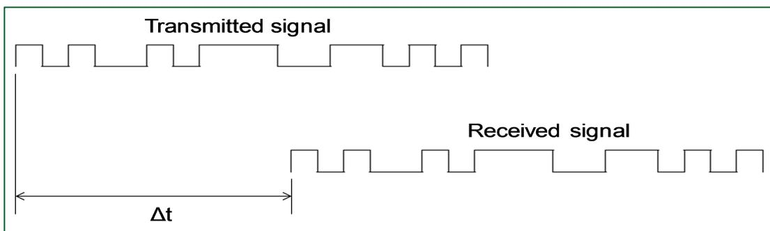
Figure 3 - Graphical representation of a pseudo-range measurement
