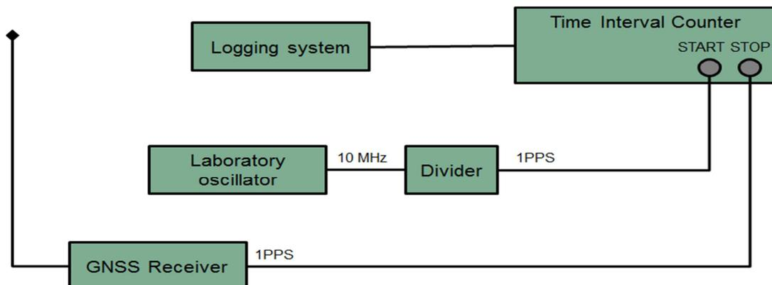
Figure 8 - Block diagram of the proposed measurement setup
