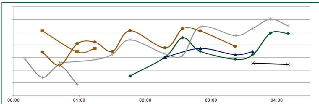
Figure 7 - GPS common-view data for two clocks (Each grid line is 10 ns)
