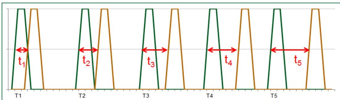
Figure 1 - Illustration of a time difference measurement between two clocks
