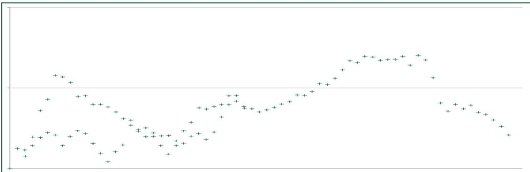
**Figure 6 - The time error of a GPS disciplined Rubidium oscillator
