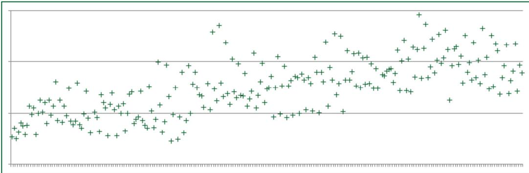
**Figure 5 - The difference between GPS and a local clock for a 24 hour period
